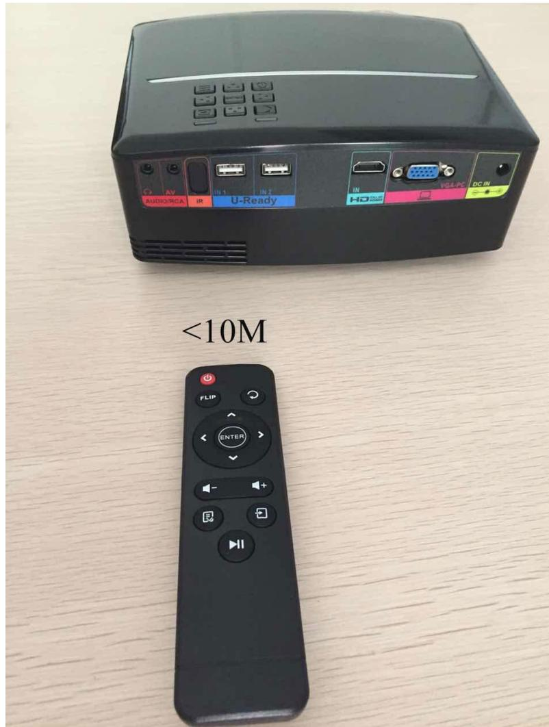
The maximum effective remote control distance of the infrared remote control is 10M. In order to ensure the sensitivity of infrared sensors, we recommend that the longest remote control distance in about 7M.
